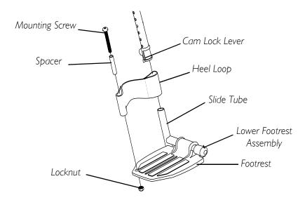
FIGURE 6.3 Replacing the Heel Loop
